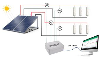
A1- Amperage meter 1; A2 - Amperage meter 2; V1 - Strain gauge 1; V2 - Strain gauge 2 **Figure 2.** Photovoltaic modules, data acquisition system and recorder (datalogger), Arduino microcontroller computer
