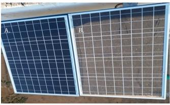
**Figure 3.** Photovoltaic modules - module cleaned weekly (A) and not cleaned, with accumulated dirt on the 177<sup>th</sup> day of the experiment (B)
