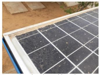
**Figure 6.** Dirty photovoltaic module: non-homogeneous, cement layer and residual dirt
