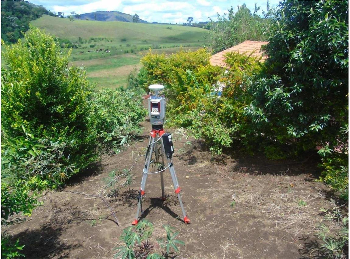
**Figure 3.** Riegl VZ-1000 TLS terrestrial laser scanner (TLS) in action, scanning the mixed-area section in the home garden of Espera Feliz
